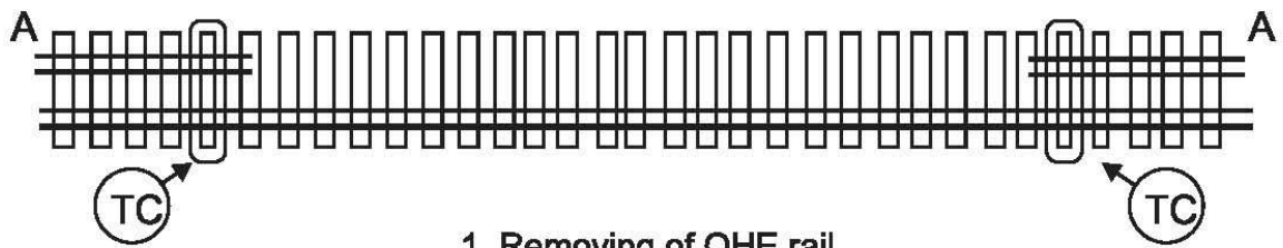
1. Removing of OHE rail Both the rails insulated for track circuiting
