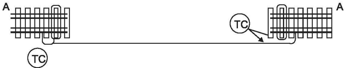
2. Removing both the rails simultaneously of OHE line Both the rails insulated for track circuiting
