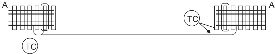
2. Removing both the rails simultaneously of OHE line Both the rails insulated for track circuiting
